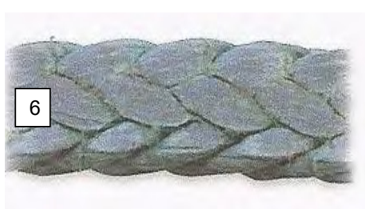
> Image 6 This rope is showing signs of compression.
